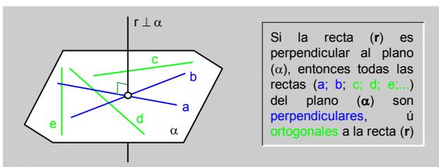
fig.169. \ Recta (r) perpendicular a un plano ( $\alpha$ ).
