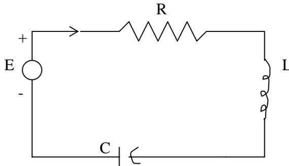
$$E_r = IR, \quad E_L = \frac{LdI}{dt}, \quad E_c = \frac{Q}{c}, \quad \frac{LdI}{dt} + Ia + \frac{Q}{c} = E, \quad I = \frac{dQ}{dt}$$
